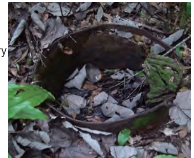
Drums found at former Landing Zone-1, soil surrounding the drums was found contaminated with PCB
