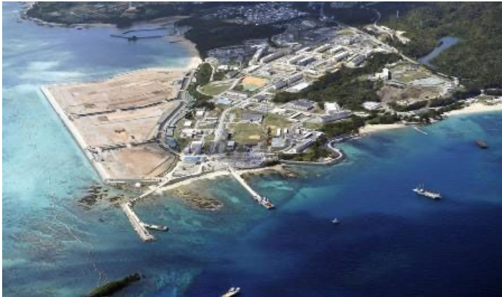
On Henoko side, land reclamation work has shown some progress. On Oura Bay side, little progress has been made due to soft seafloor. Image Source: Kyodo News
