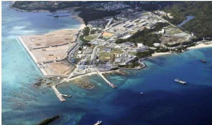
On Henoko side, land reclamation work has shown some progress. On Oura Bay side, little progress has been made due to soft seafloor. Image Source: Kyodo (April, 2022)
